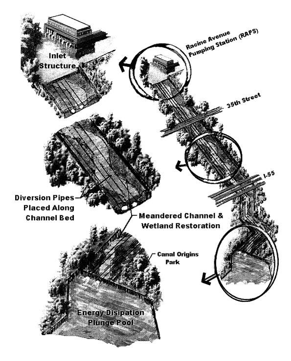
*Figure 6*: Low-Flow Restoration, Combined Sewer Overflow Elimination, and Sediment Remediation with Ecosystem Restoration Preliminary Plan
